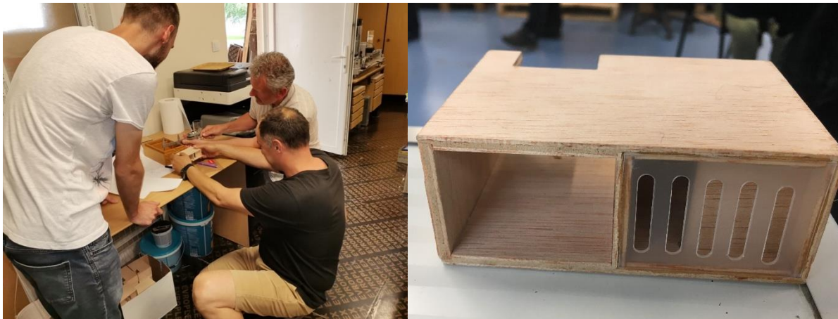
Figure 17. Manufacturing of the labyrinth. Dr Dahle and Dr Uzunov (middle, right) are testing the fitting of the labyrinth in to the mating nuc (left pane). Manufactured wooden labyrinth prior to its embedding into the mating nuc. Left-side corridor is a pass-through allows direct light access for permitting nuptial flight, which is normally closed during the day. The right-side corridor is constructed as a labyrinth to block the light but allow normal traffic for worker bees. Queen is prevented exit by means of small queen excluder (right pane).
